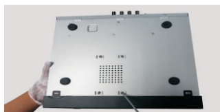
④ Turn over the machine and secure the HDD with the screws.
